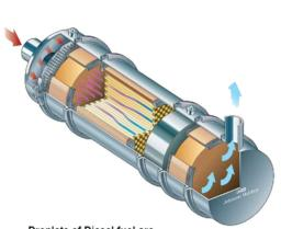
Droplets of Diesel fuel are injected between the filter and an additional decomposition catalyst to reduce NO2 levels. A filter monitor controls the injection rate depending on the exhaust gas temperature and the engine speed. This system reduces 99.8% of the number of particulates, 90% of the CO and HC, and NO2 is kept at the engine out level.
